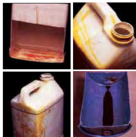
Containers caked with residue, dried formulation on container and thread or liquid residue present.
